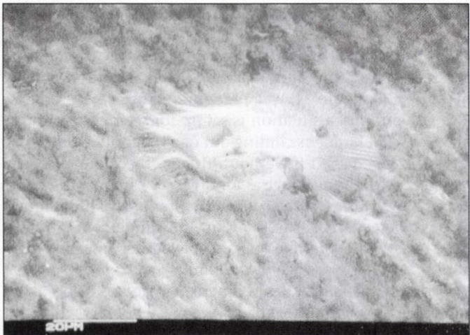
Figure 10. Backside of a 6 micrometer thick aluminum foil struck with an EV and a deposit of aluminum oxide.
