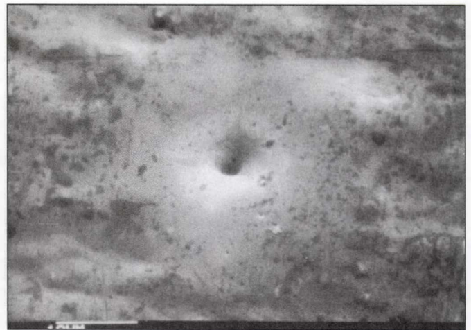
Figure 2. EV strike on 6 micrometer thick aluminum foil. Exit side.
