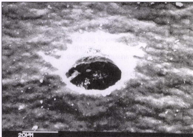
Figure 13. Exit side of an EV strike on silicon carbide grain coated on a 0.001" thick aluminum foil.
