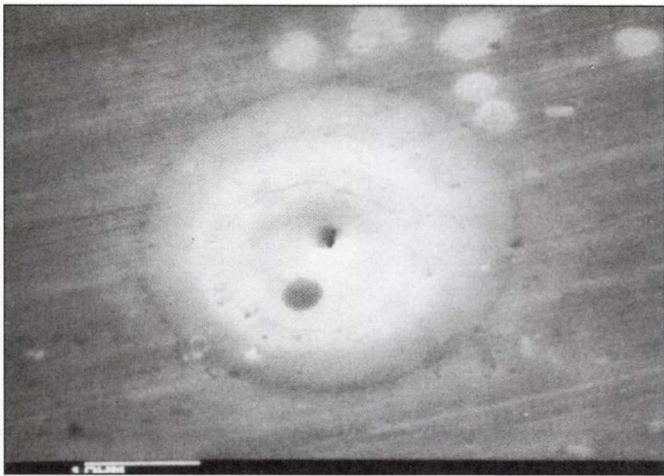
Figure 1. EV strike on 6 micrometer thick aluminum foil. Entry side.
