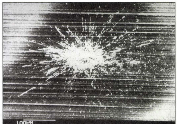
Figure 14. Single shot of silicon carbide ejected from a borehole into a foil of aluminum.
