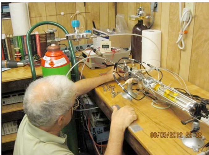
Celani charging the reactor with hydrogen at LettsLab in Austin, Texas, before NIWeek demo. (Photo by Dennis Letts)
