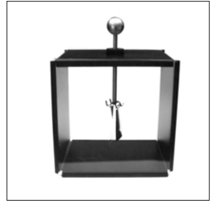
A simple, commercially available leaf electroscope.
